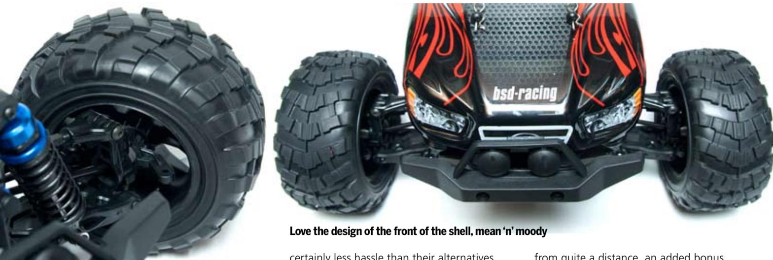
**Note that the steering knuckles are moulded symmetrically, so less spares required**
