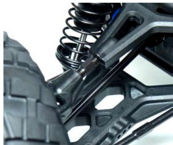
Turnbuckles are built into the upper arms and linkages, this means one thing... TUNING!
