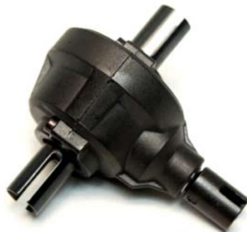
The diff's each end fit into casings that are then held in place within the bulkheads
