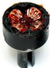
Diff's are hardened steel, planetary type and packed with grease
