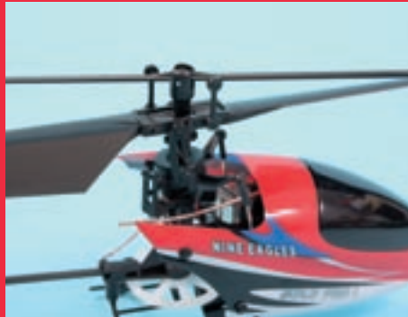
Close-up of the clever Bell-Hiller control mixing arms on the Nine Eagles patented rotorhead
