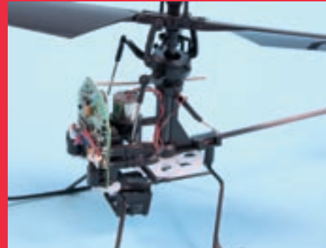
Under the canopy you will find a simple plastic main frame and the 4-in-1 electronic controller
