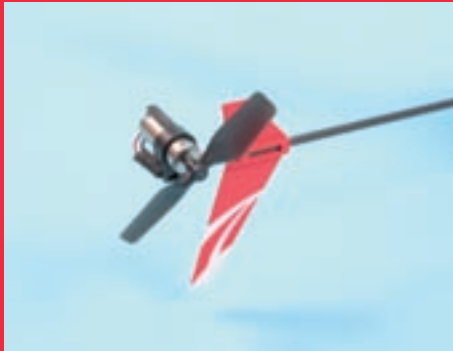
The Solo also features a tiny little 6mm micro motor to drive the tail rotor that gives rudder control
