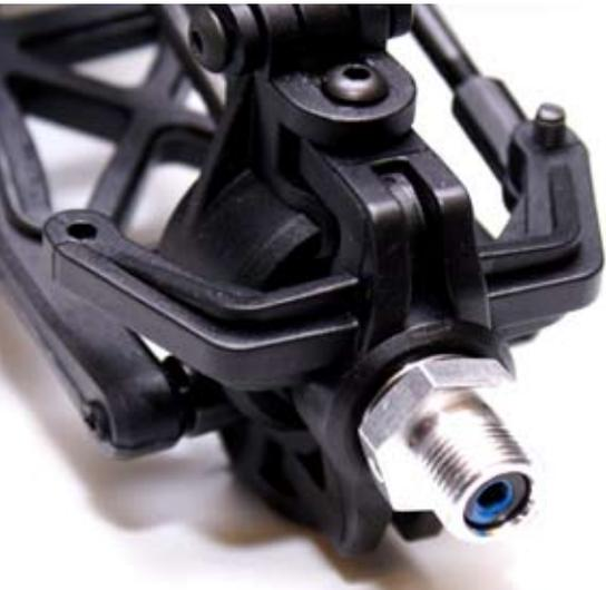
**Note: the steering knuckles aren't handed so less spares are required**
