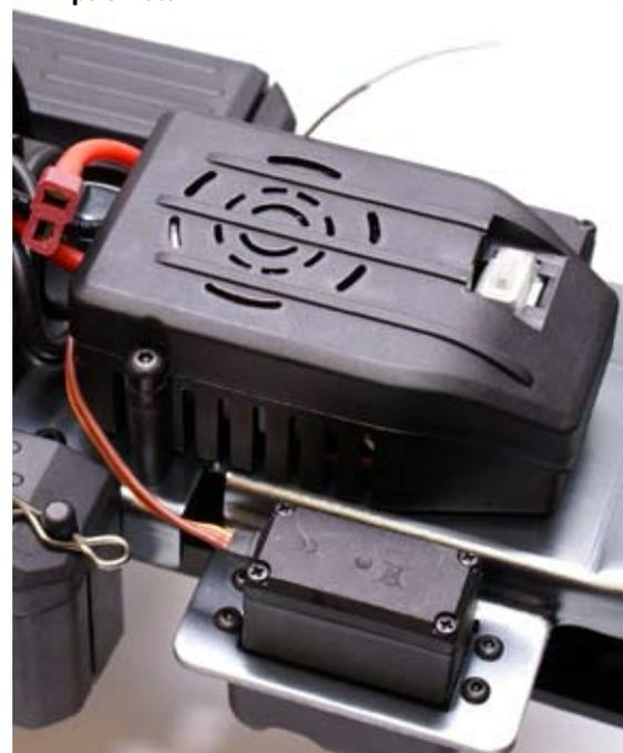
How's that for a neat place to put the ESC and receiver?
