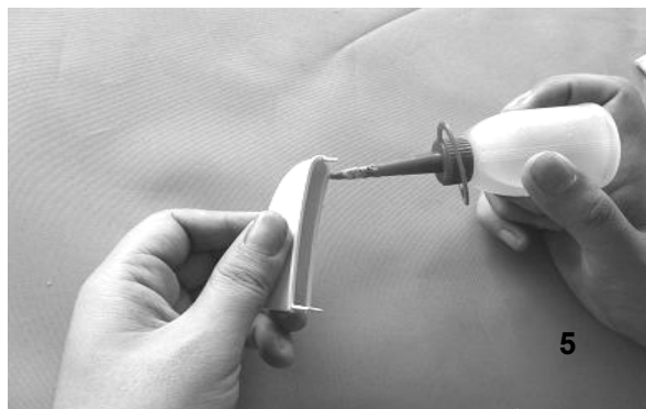
Fig. 5 - Glue the servo fairing.
