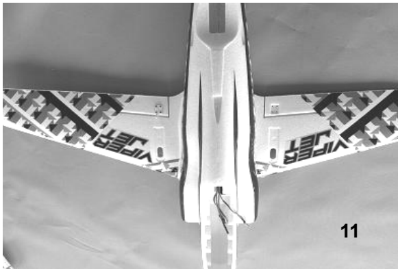
Fig. 11 - Thread the aileron servo lead up through the fuselage and into the receiver bay before gluing the wings in place.
