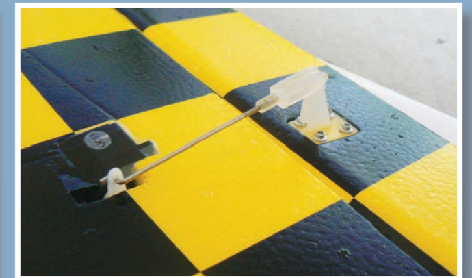
Servo links to the ailerons are short and stiff - perfect!
