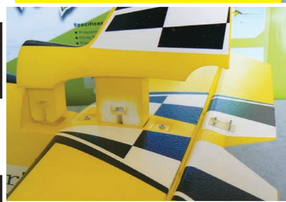
Tail assembly simply bolts in place - very much akin to the excellent Riot reviewed a couple of issues back!
