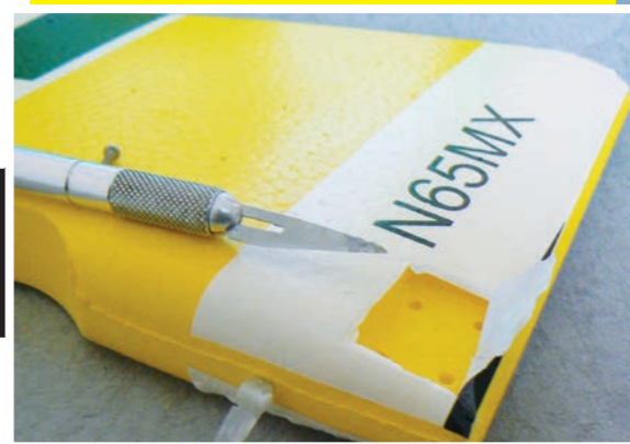
This area needed relieving for the control horn.
