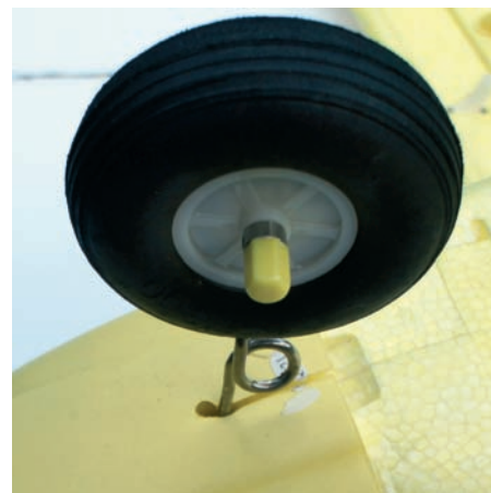
Big wheels make rough grass take-off and landings easy. I fitted a metal collet behind the plastic nut to cure some nose wheel wobble
