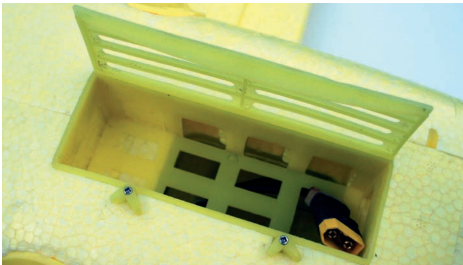
The battery compartment is designed for a 3S 1800 but I got a 3S 2200 to fit. It's a bit tight though
