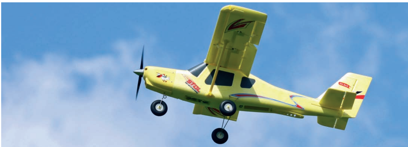
The model handles really well when the flaps and slats are down. Slow speed flight really is slow, particularly if there is any headwind
