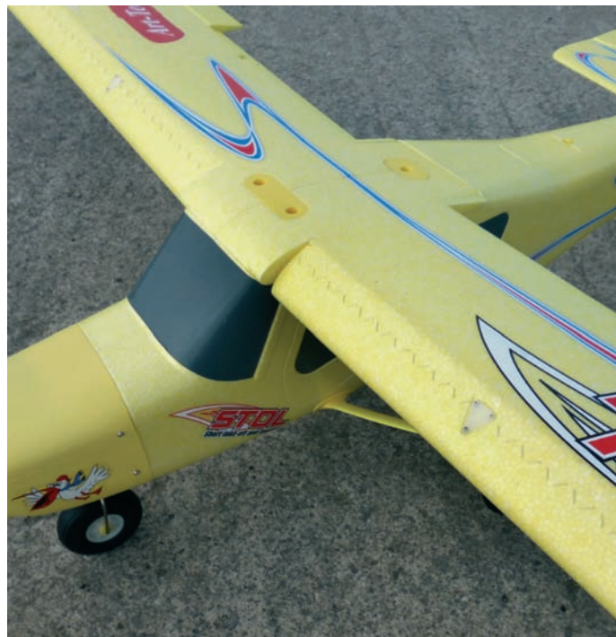
The slats droop by a noticeable amount. Stress cracks that formed on the slat hinge were easily fixed with Blendederm tape
